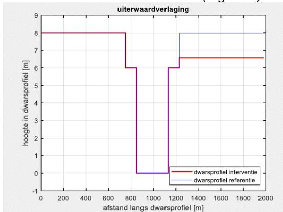
Figure 2. Example measure flood plain lowering
