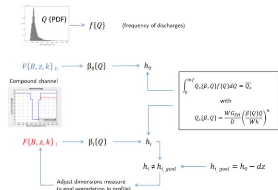
Figure 1. Flow diagram for the inverse analytical method
