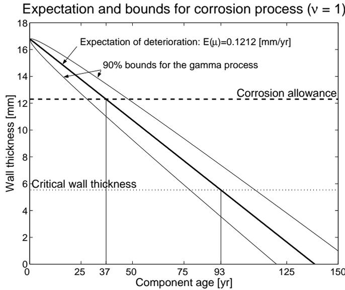
Fig. 4. Expectation and 90% confidence bounds for the gamma process using the posterior expectation of the average corrosion rate  $\mu$ .
