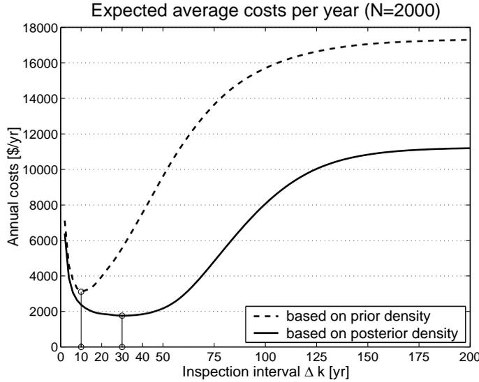
Fig. 3. Expected average costs per year for the hydrogen dryer.
