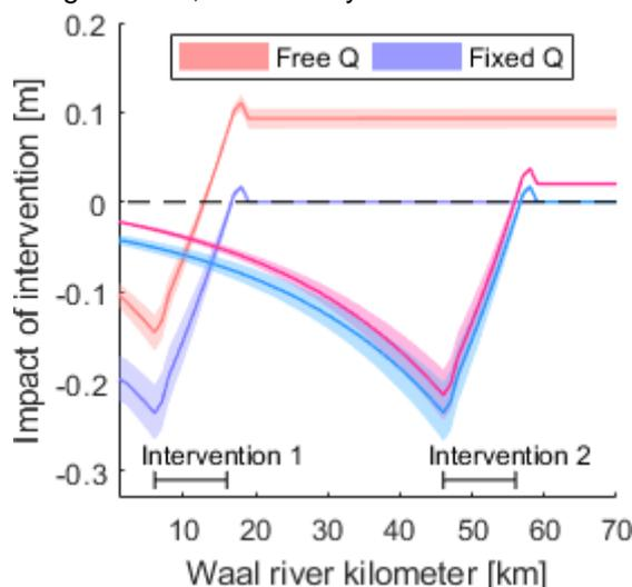
Figure 3. The impact on water levels along the Waal branch of interventions with upstream kilometres 6 (intervention 1) and 46 (intervention 2) if the discharge distribution ( $Q$ ) is free (red) or fixed (blue). The bifurcation point is at km 0. The continuous line gives the mean impact, while the shaded area indicates the 90% confidence interval.
