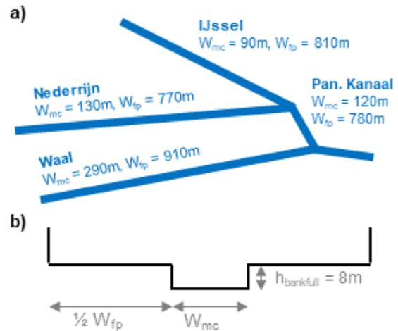
Figure 1. a) Schematization of Dutch Rhine branches and b) the geometry of the compound cross-sections.  $W_{mc}$  and  $W_{fp}$  are the width of main channel and floodplain respectively.
