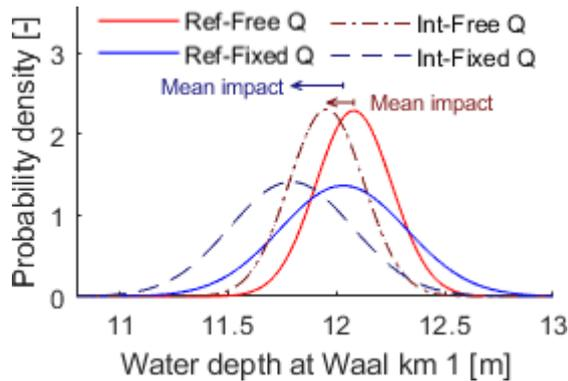
Figure 2. Probability density functions for the water depth at Waal km 1 in the reference and in the intervention model for both a free and a fixed discharge distribution ( $Q$ ). The upstream end of the intervention is at km 1.
