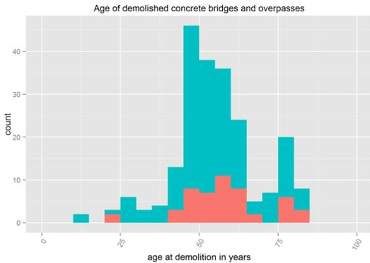
Figure 4: Distribution of structures' age at demolition. Bridges in green. Overpasses in red.
