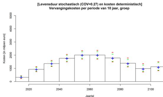
Figure 9: Expected future replacement costs of concrete structures as a function of time based on model 3. The red dashes (-) are 5<sup>th</sup> and 95<sup>th</sup> percentiles, the green dashes (-) are 10<sup>th</sup> and 90<sup>th</sup> percentiles, and the blue pluses (+) are the 50<sup>th</sup> percentiles.
