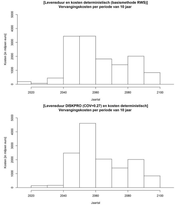
Figure 7: Expected future replacement costs of concrete structures as a function of time based on methods 1 and 2 (from top to bottom).
