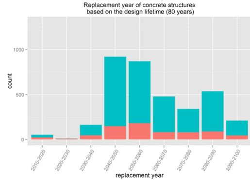
Figure 2: Replacement year of concrete structures based on the design lifetime of 80 years. Bridges in green. Overpasses in red.
