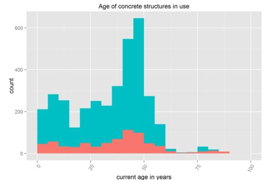
Figure 3: Age distribution of concrete structures in use. Bridges in green. Overpasses in red.
