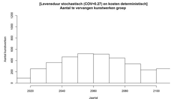
Figure 8: Distribution of the replacement year of concrete structures based on the structures' posterior lifetime distributions (models 3 and 4). Replacements beyond the year 2100 are added together.
