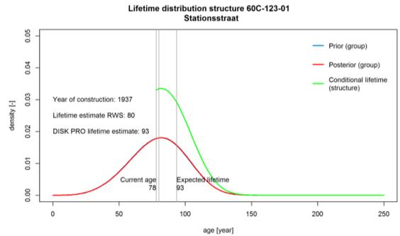
Figure 5: Generic lifetime distribution of concrete structures (red line) and (remaining) lifetime distribution of a particular bridge (green line).
