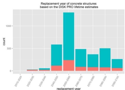
Figure 6: Replacement year of concrete structures based on the structures' DISK PRO lifetime estimates Bridges in green. Overpasses in red.
