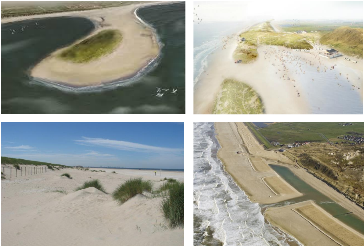
Figure 6. Upper Artist impressions with vegetated dunes for the Sand Motor (left) and the HPZ (right). Lower: Natural dune development at the Sand Motor (left) using the existing dune system as a basis versus artificial constructed and planted dunes at the HPZ (right).
